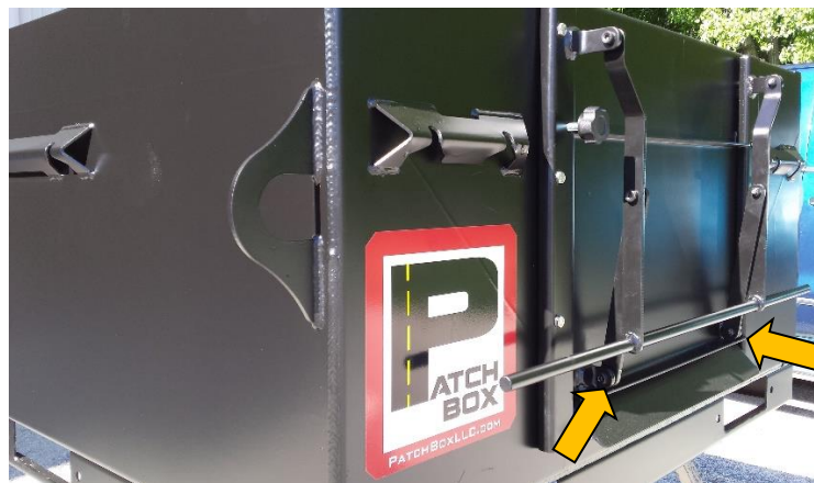
Figure 8 – Removing door if equipped with the Door Linkage Kit Option
