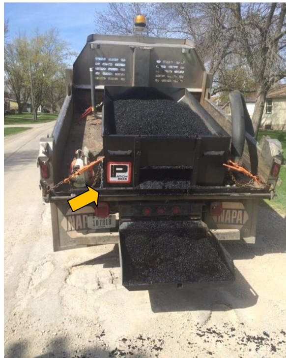
Figure 1 – Ratchet binders with downward force are recommended for securing PatchBox Note removable metal plate used as redundant stop (see arrow)
