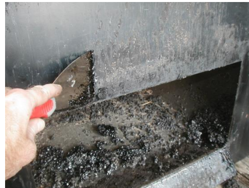
Figures 6 & 7 – Cleaning back of the door and surface above the door
